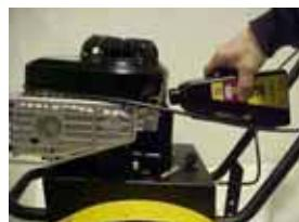
Remove the spark plug. Pour a couple of drops of motor oil down the spark plug hole. Pull the start cord 4-5 times and replace the spark plug. Pull the start cord slowly until you feel some resistance. This closes the fuel and exhaust valves and prevents corrosion in the cylinder.
