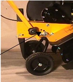
The supportwheels are mounted on the cultivator. The adjustment is done by means of the lock . Pull the lock out, and lift or lower the cultivator with the handlebar until the preferred height is found. Release the lock.
