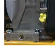
Drain the remaining of the gasoline from the fuel tank, start the engine and let it run until the residue of fuel in the carburettor has been used up and the engine stops.
