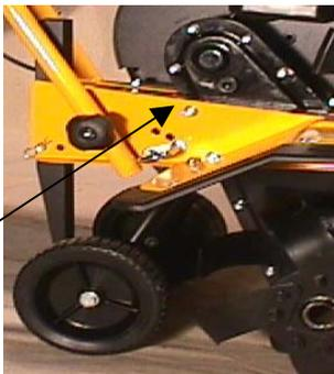
The gearbox on the cultivator is from the factory lubricated with 0.2 litre TEXACO Multifak 283 EPOO oil. It is not necessary to renew the oil
