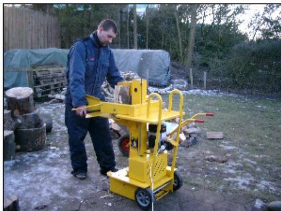
Variable splitting length from 10-105 cm. Height is adjusted by pushing down both handles (vertically) to the requested size of wood. Here you let go of one of the handles (shown with arrow) Loosen the knurled nut (shown) and the bar indicating the height is pulled up and the knurled nut is refastened (shown).
