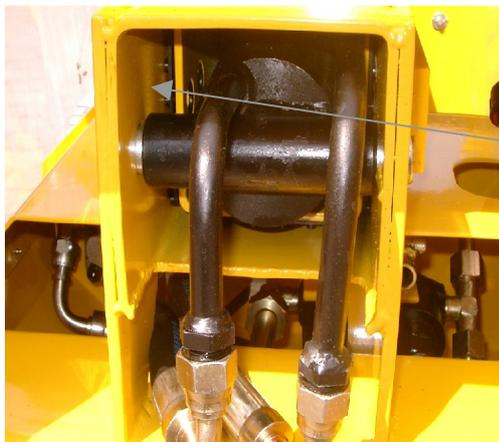
Lubricate with some oil in the piston tunnel on all 4 sides.
