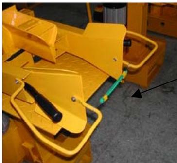
The strap can fasten the handles during transport.
